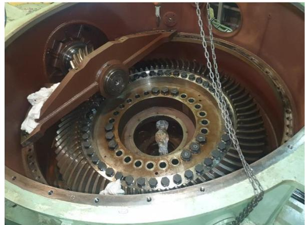
Figure 2: Inside the equipment room – Here: The Voith Schneider Propeller gearbox ready for service.
