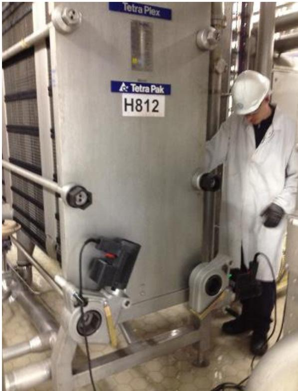
Figure 2: alkitronic radial torque multiplier in use.
