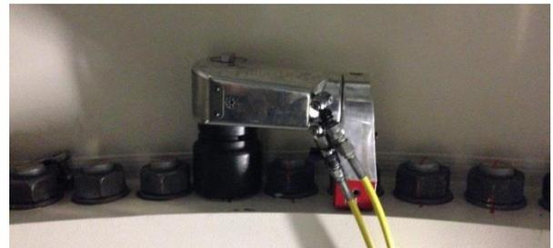
Figure 5: alkitronic® Hydraulic torque wrench AS-15 on tower flange bolts M64- high tension
