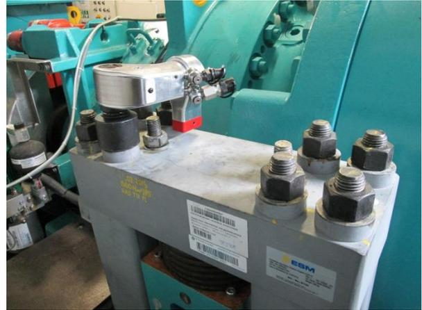
Figure 3: Hydraulic torque wrench AS-3 on pedestal bearing
