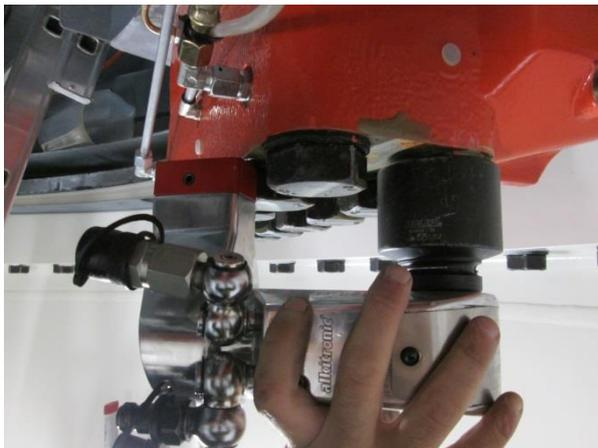
Figure 2: alkitronic® AS-3 overhead on an azimuthal brak
