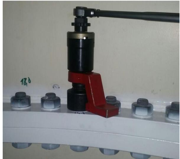
Figure 8: alkitronic® Manual torque multiplier HG 20 on tower bolts M36- high tension
