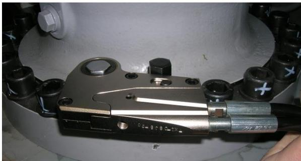
Figure 7: alkitronic® Hydraulic torque wrench AX-1 up to 750 Nm on azimuth drive
