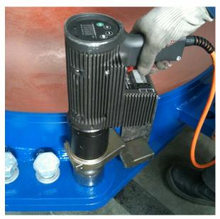
Figure 3: Der alkitronic EFCip 70 in use for the mosque in Algiers. Photo courtesy: Maurer Söhne GmbH
