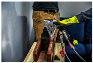
Figure 1: alkitronic<sup>®</sup> AS 3 Hydraulic torque multiplier in use during training
