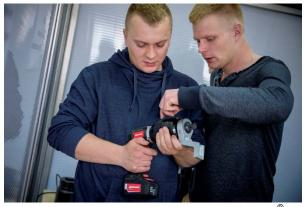
Figure 3: Training participants with an alkitronic<sup>®</sup> Battery torque multiplier EA 2/80
